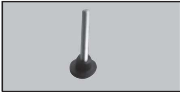
Control horn of Aileron
